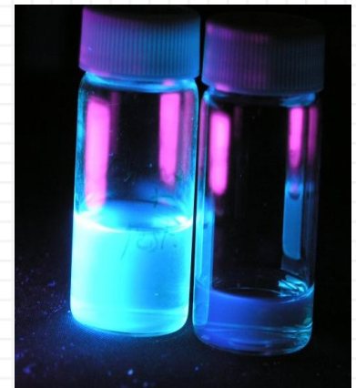
Figure 1: The image on the left shows two vials of the NDSU compound under white light, one containing a poison and one containing a "clean" liquid. The image on the right shows the same liquids when viewed under ultraviolet light. The liquid containing the poison and the sensing compound fluoresces, indicating the presence of a poison.
